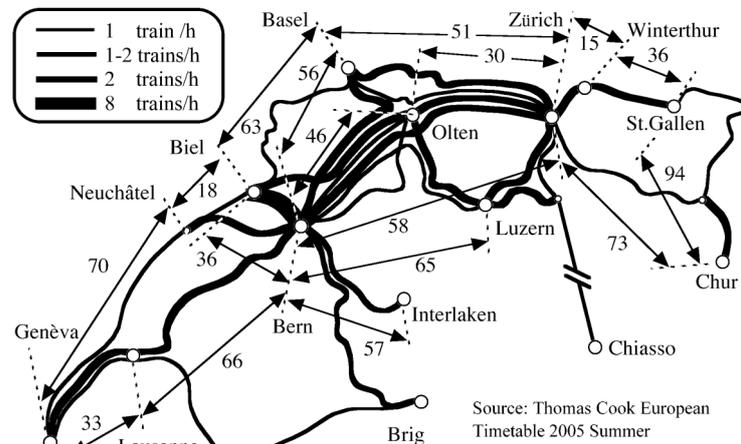
**Figure 2 Train Frequency and Block Time in Switzerland**
