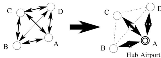
Figure 7 Hub System of Airline Network
